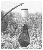
Figure 3.10. Battery-operated CDC Miniature Light Trap
